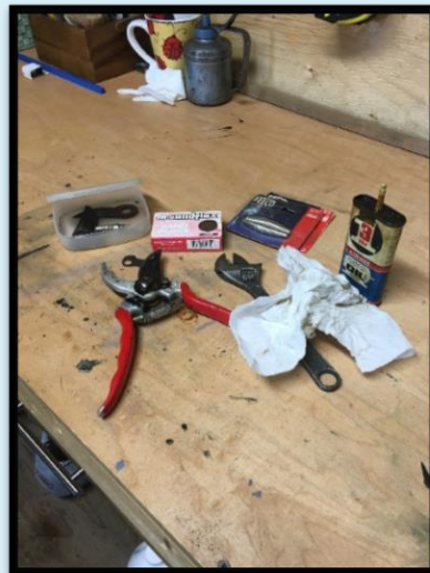
These secateurs are getting a make-over, new blades, springs, and a good buffing with a rust pad.
